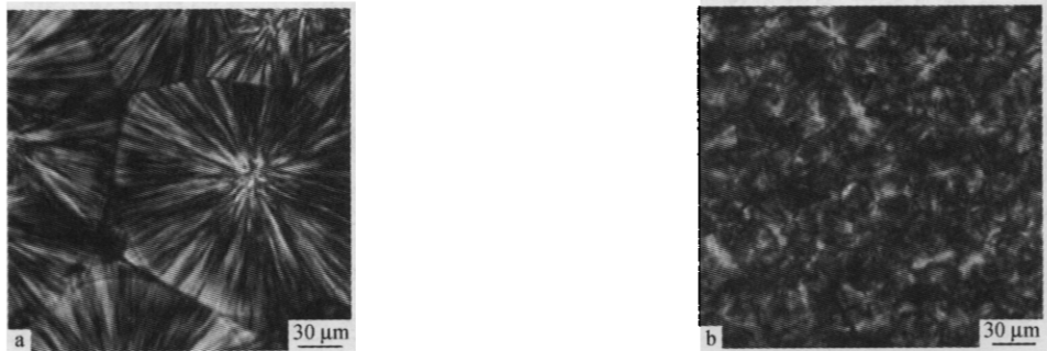
Fig. 4 POM photographs of pure PP (a), PP/ATP(ATP content 5%, mass fraction)(b)
